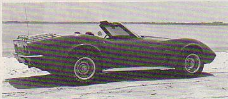
Last year for the chrome rear bumpers. If there's a chrome bumper on the back but none on the front, then you know it's a '73. This gives the '73 an individual identity that most other Corvettes lack.
