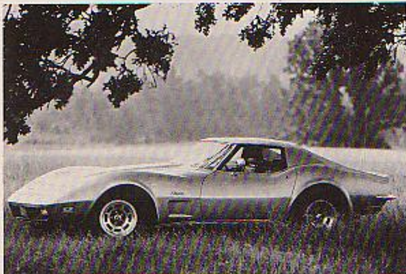
Virtually unchanged since 1968, '73 Corvette is revamped substantially to meet federal safety requirements; comes off cleaner than the original version in the process. Grill-less side vents, new nose and hood bulge account for major changes. New alloy wheels reduce unsprung weight by 40 lbs.
