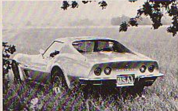
Virtually unchanged since 1968, '73 Corvette is revamped substantially to meet federal safety requirements; comes off cleaner than the original version in the process. Grill-less side vents, new nose and hood bulge account for major changes. New alloy wheels reduce unsprung weight by 40 lbs.
