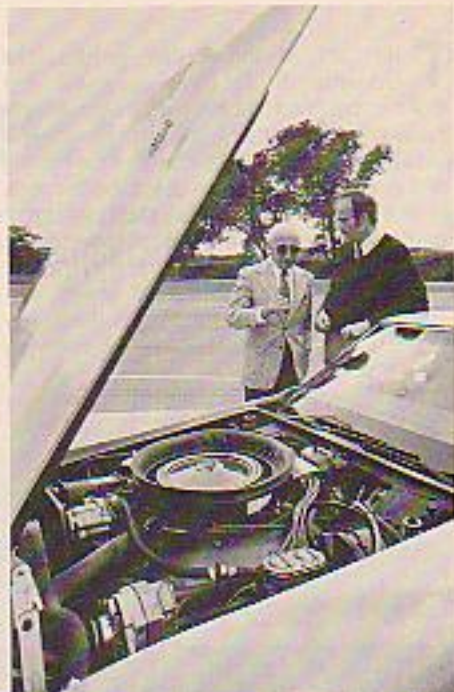
Above: Zora Duntov (in sunglasses), explains the intricacies of revitalized LS-4 engine for 1973. Cold-air, cowl-induction for carburetor has improved performance and lowered emissions at the same time.
